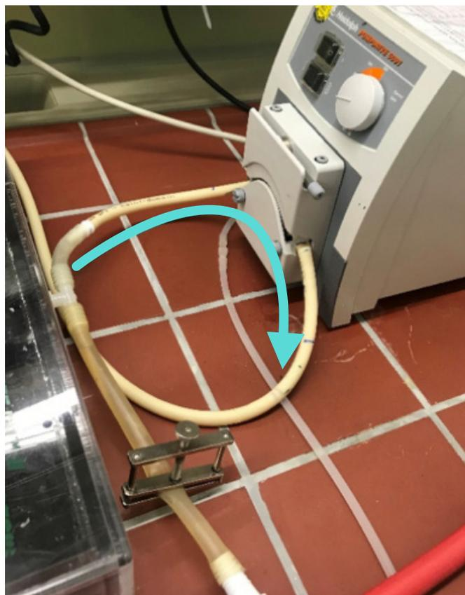
**Fig. 4:** The connected pump with the PharMed® tubing. Also shown is the flow or pump direction of the running buffer.
