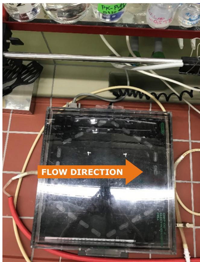
**Fig. 2:** Top view on the gel chamber, the flow direction of the buffer solution is indicated by the red arrow
