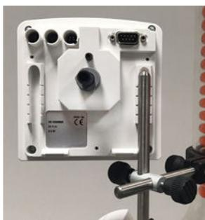
2. Attach the support rod to the evaporator and attach the controller to the top end of the support rod, so that the support rod locks into the gap on the back of the controller.
