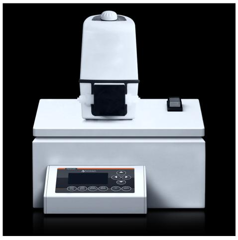
You can use the control panel on the control box of the Hei-VOLUME Distimatic 24/7 module to enter the parameters for the sensor or time-controlled filling of the rotary flask. The emptying times of the coated collector vessel (approx. 400 ml) and the residue from the rotary flask by the two chemical membrane pumps can also be programmed. The control box can be mounted on a nearby wall using the supplied bracket with hose guide.
