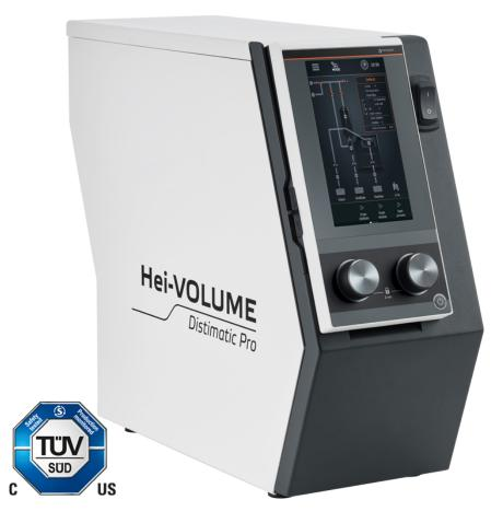
For high-performance distillation with the best separation performance, suitable for most solvents (A1 version), also when processing foaming media (A2 version): Version with adapter for Hei-VAP Industrial with glassware of the A series (A1, A2)
