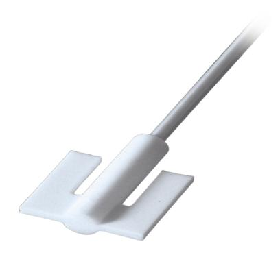
Particularly in applications with very viscous media, it is important to have a stirring tool in use that enables the mixing process up to the edges of the vessel. This explains the shape of the anchor-type impeller and the width of the stirring blade of 60 mm.
